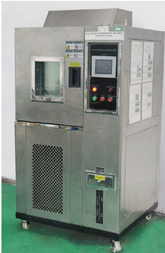
Climate chamber, with temperature adjustment range from -90 to +150^\circ\text{C} , relative humidity adjustment range 1 to 100%
