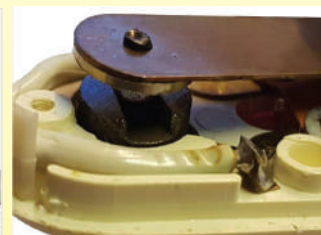
1972 ca. Power control box made by Jidé in Limoges under the brand Jidéstat. The most successful of all systems. Very small in size, it is adjustable, and is incorporated in the electrical plug. This is the only model with a snap magnet contact. It was not surpassed by electromechanical systems until the current era. (Ultimheat Collection)
