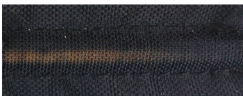
1h at 220°C on the heating cable: the PA66 starts to change color
