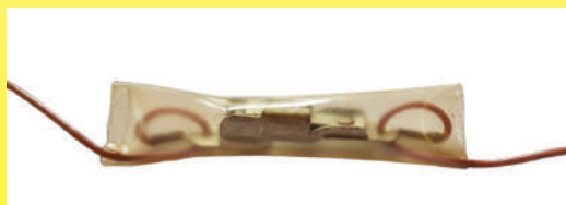
Calor slow-break heating blanket temperature limiter, calibrated at 80°C (circa 1960). Note the waterproof PVC sleeve welded on the wires and the loop made by the electrical conductors passing through a hole in each terminal- this is to eliminate tensile stresses on the wire (Ultimheat Collection)
